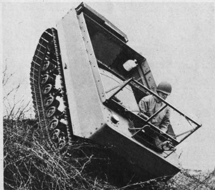
Agile on land as well as water, the M-29 can negotiate almost any grade. Weasel's large capacity is apparent in the open-topped box hull.
